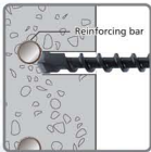
Torque Limiter When drill bit hits against reinforcements, Torque Limiter operates to stop.
