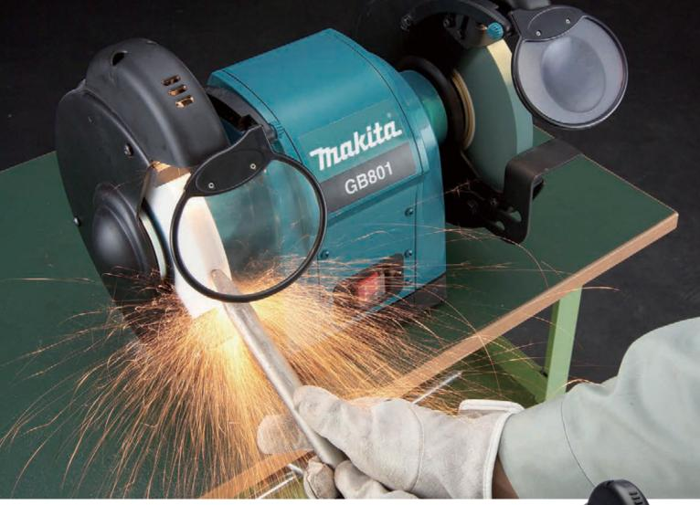
Ideal for sharpening tools and for removing rust or corrosion
